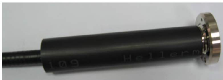
Picture 17.: Shrinking tube over the connector
