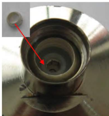
Picture 11.: inserting the inner ring in to the main body
