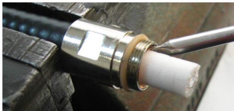
Picture 7.: smoothen the edge of the cooper shield
