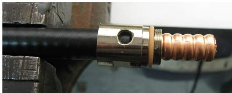
Picture 3.: Cable with the body of the connector
