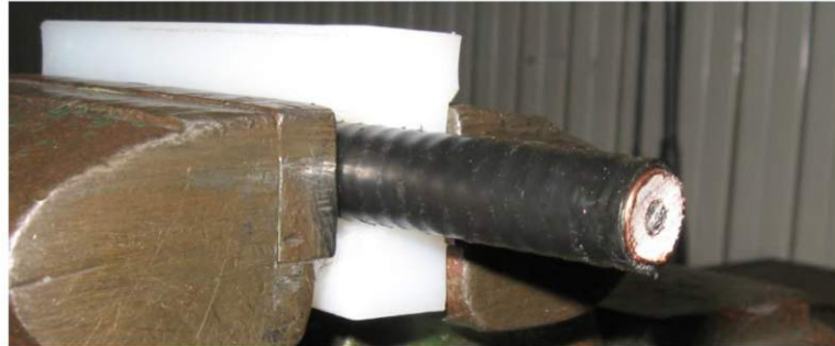
Picture 1.: Even cut off cable
