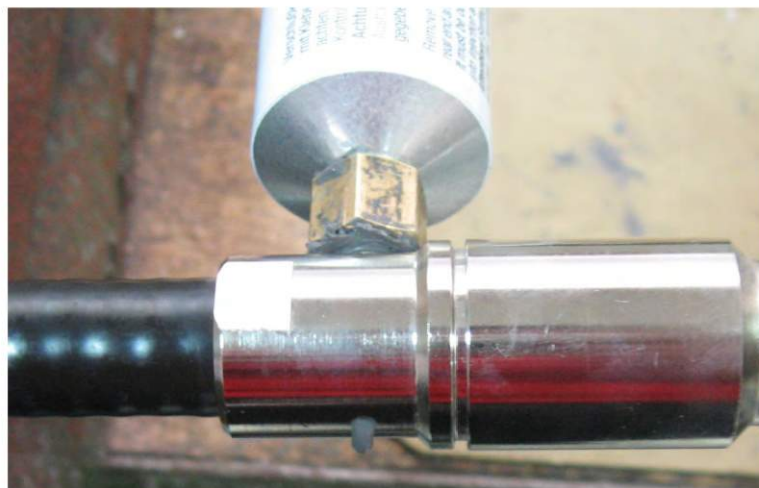
Picture 14.: The connector filed up with the past
