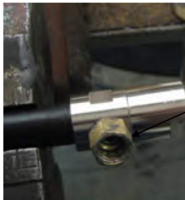
Picture 13.: connector with the adapter for the PLAST 2000
