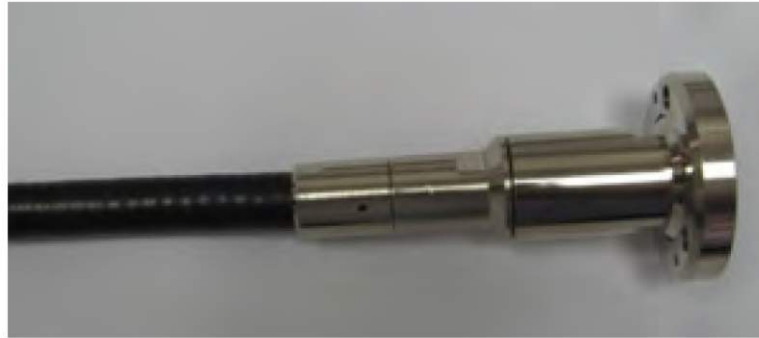
Picture 12.: assembled connector on the cable LCF 1/2
