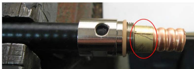
Picture 4.: Cable with contact ring
